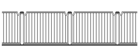
DECORATIVE FENCE DETAIL OPTIONAL WOOD FENCE PANEL 8' WOOD FENCE PANEL TO BE INSTALLED BETWEEN PATIOS AS SHOWN FOR PRIVACY, AND ROAD FRONTAGE WHERE SHOWN.
