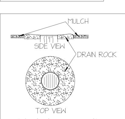
DRAINS IN SHRUB BEDS SHALL HAVE A 600mm (24") DIAMETER RING OF DRAIN ROCK 100mm (4") DEEP AS A BARRIER FROM THE BARK MULCH, TO PREVENT MULCH FROM GOING DOWN THE DRAIN.
